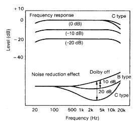
With cassette tapes, the most noticeable form of noise is high frequency hiss. T reduce this hiss noise, this unit is equipped with the older Dolby B noise reducti system in addition to the newer Dolby C NR. Either type of noise reduction may selected with the DOLBY NR selector.
